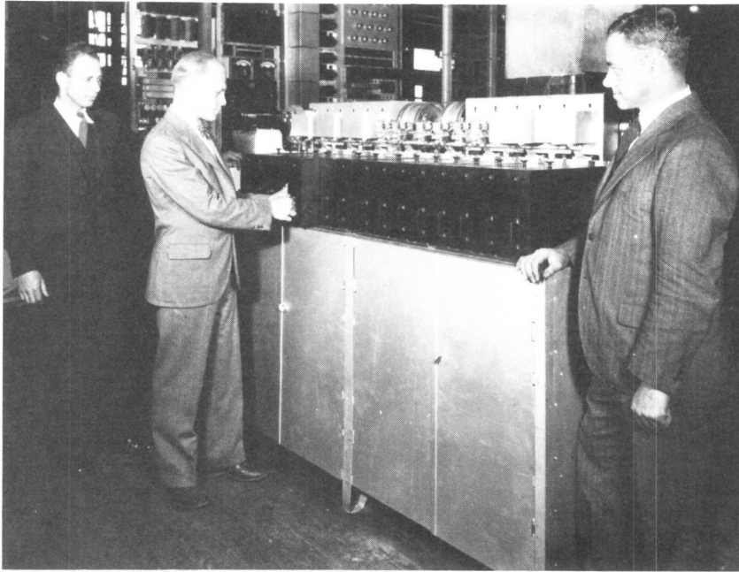
Fig. 3-11. Call announcer system using sound-on-film to produce voice announcements of dialed numbers. Left to right: C. J. Beck, F. K. Low, and C. C. Towne.
