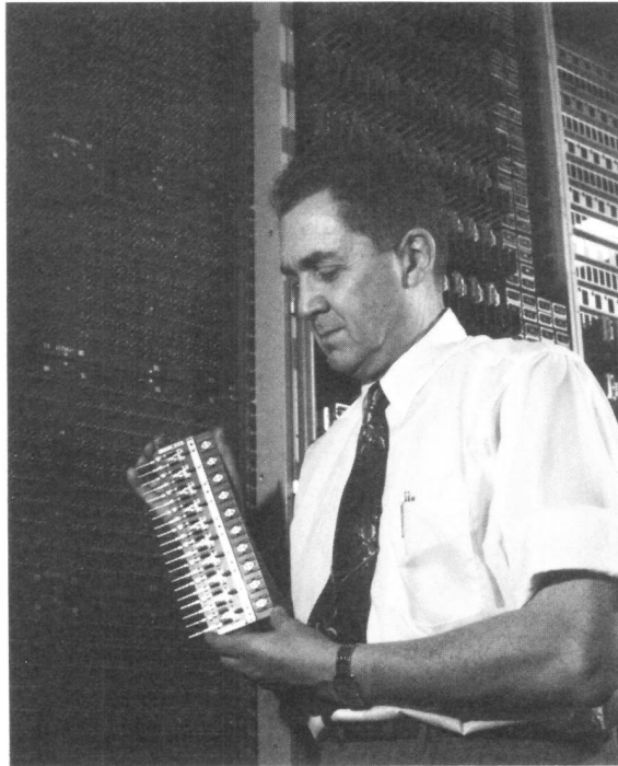
Fig. 6-29. H. A. Miloche standing in front of an ANI-B number network frame that serves 1000 lines. He holds a primary network unit for ten telephone lines.
