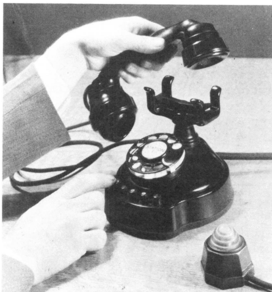
Fig. 13-53. Pushbutton handset used with 15A and 23A key telephone equipment (early 1930s). Buttons accessed central office and intercom lines, put calls on hold, and signaled other telephones.
