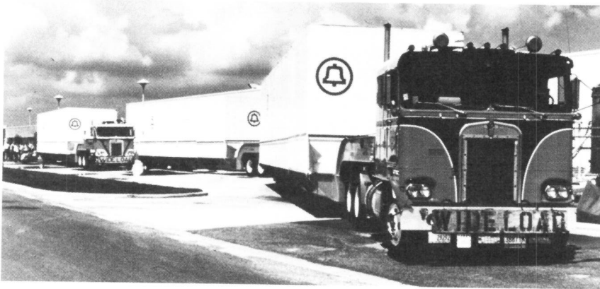
Fig. 9-71. Transportable No. 2A ESS. Units are assembled at the factory with connectorized cables. Set on a precast foundation, system quickly provides service for 3000 lines.
