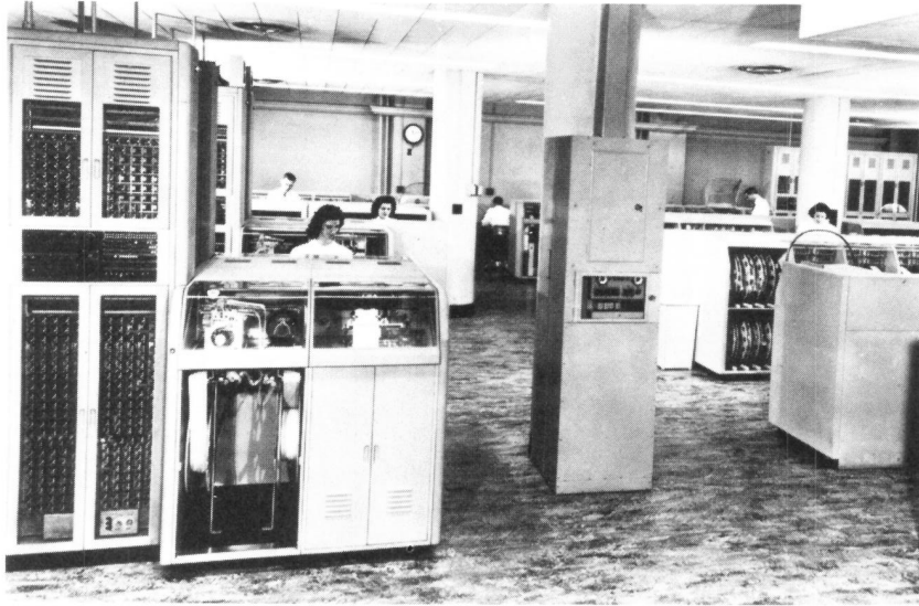
Accounting center in Philadelphia, 1948, equipped to process automatic message accounting (AMA) tapes. AMA centers, installed in the Bell System from 1948 to 1963, were an important first step toward the eventual complete automation of telephone billing. A wide AMA paper tape recorded the calling and called numbers, trunk number, type of billing, and times of beginning and end of each call. Such data were entered as perforations in the paper, rather than as die-cut punched holes as in teletypewriter tape. At accounting centers the tapes were read by machines that produced monthly bills for customers.
