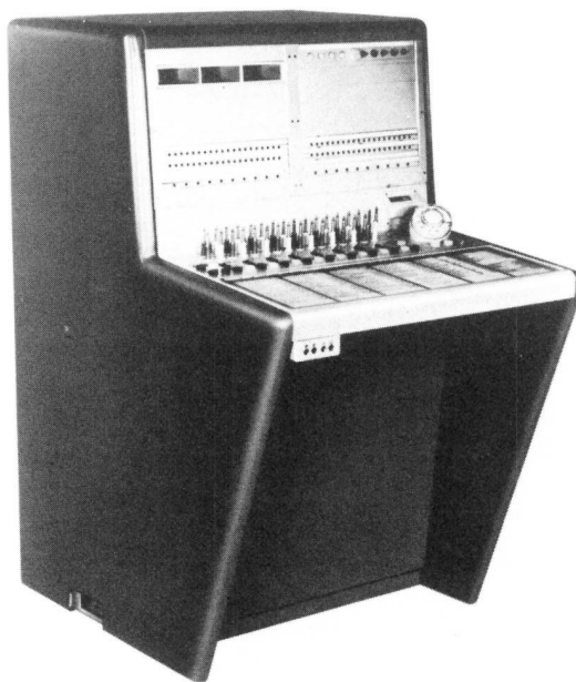
Fig. 13-11. The 608A switchboard, serving from a few telephones to as many as 2400. The 608A was the last new cord switchboard to be designed in the Bell System.
