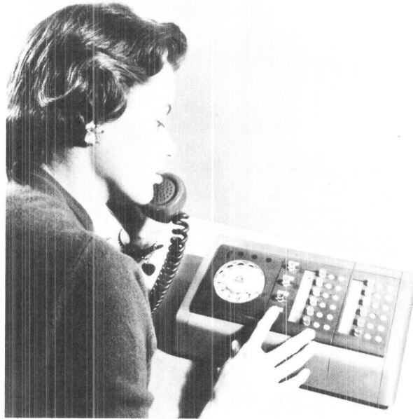
Fig. 13-10. Cordless attendant position for the 756 PBX. Its simplicity of operation set a pattern for a subsequent line of consoles.
