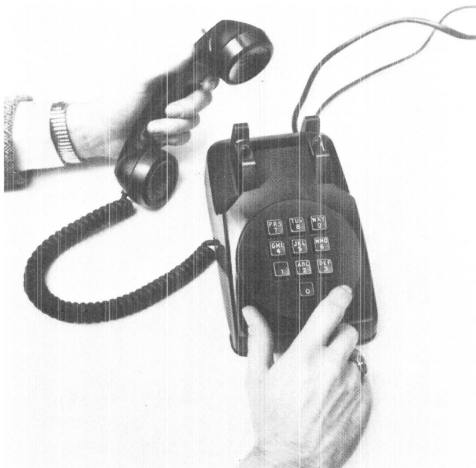
Fig. 11-2. Experimental pushbutton telephone using transistor circuits to send multifrequency dial signals to the central office.
