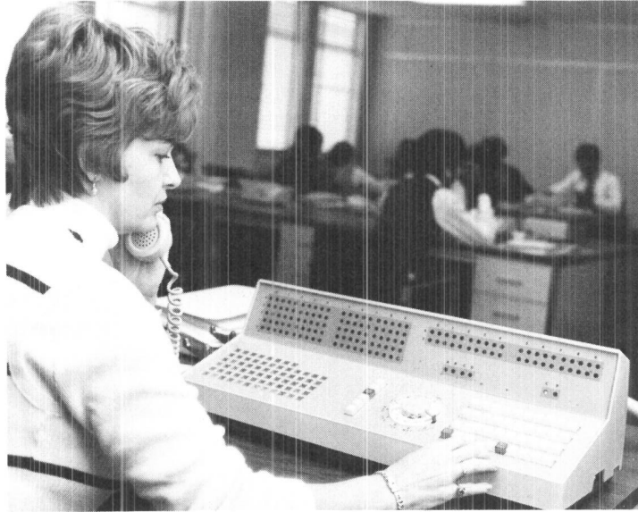
Fig. 13-75. Supervisor's console for the 2B automatic call distributor, introduced in 1973.
