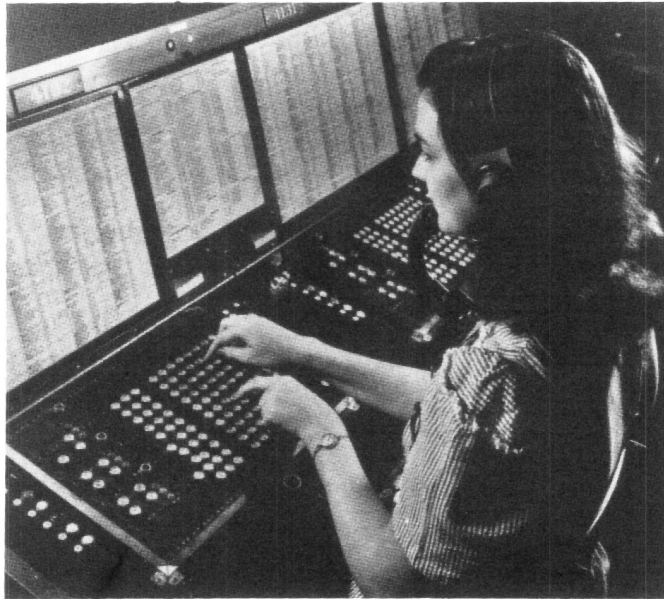
Fig. 4-18. No. 4 cordless switchboard, which separated operator functions from switching equipment.
