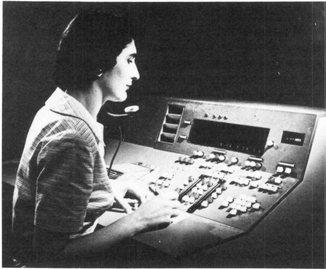
Fig. 10-2. Early (1960) model of cordless switchboard developed in anticipation of increased customer dialing of person-to-person, collect, and coin-phone toll calls.
