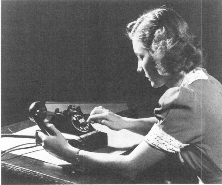
Fig. 13-56. A 300-type telephone set forming part of the 1A key telephone unit.
