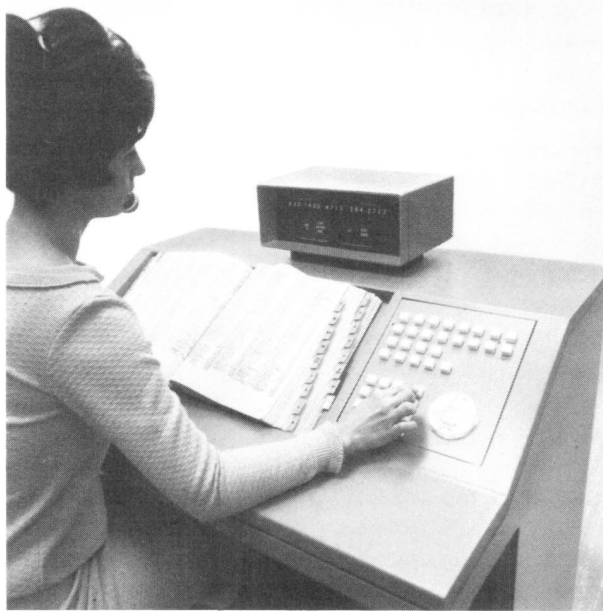
Fig. 10-16. Model of operator position used as backup to automatic intercept system. AIS was introduced into service in 1970.
