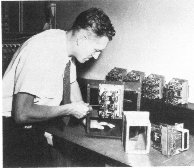
Fig. 5-21. R. H. Gumley adjusting relays sealed in containers as part of studies of contact reliability in controlled environments.
