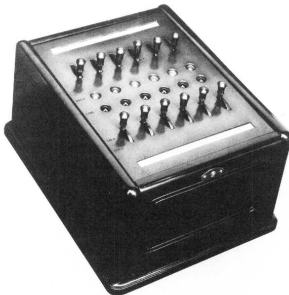
Fig. 13-51. Double-sided six-line keybox of the No. 100 key equipment. Two people seated opposite each other could access any of the six lines, and could place calls on hold.
