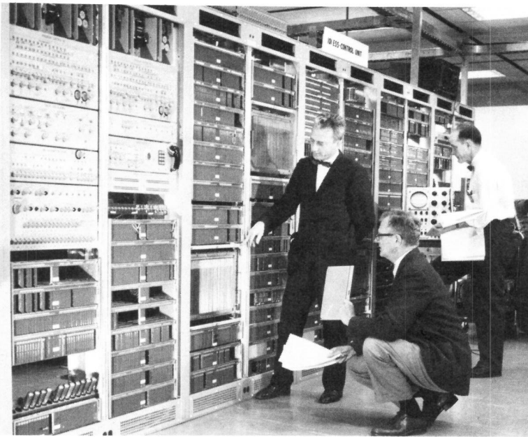
Fig. 13-13. Control unit of the No. 101 ESS. Left to right: M. A. Townsend and W. J. Means checking memory element, while H. F. Priebe checks line data circuits.
