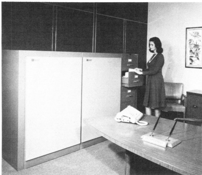
Fig. 13-21. Cabinets of the 800A electronic PBX were sized to blend with office files. ( Communications Présentées au Colloque International de Commutation Electronique , Paris, March-April 1966.)
